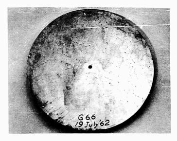
Fig. 2.14--Surface pattern of indentations from nonuniform pulse; the test plate is aluminum alloy, 20 in. in diameter by 1 in. thick; the attenuator was 4.2 lb/ft<sup>3</sup> Styrofoam; and the HE was A-3, bottom-wick-detonated
