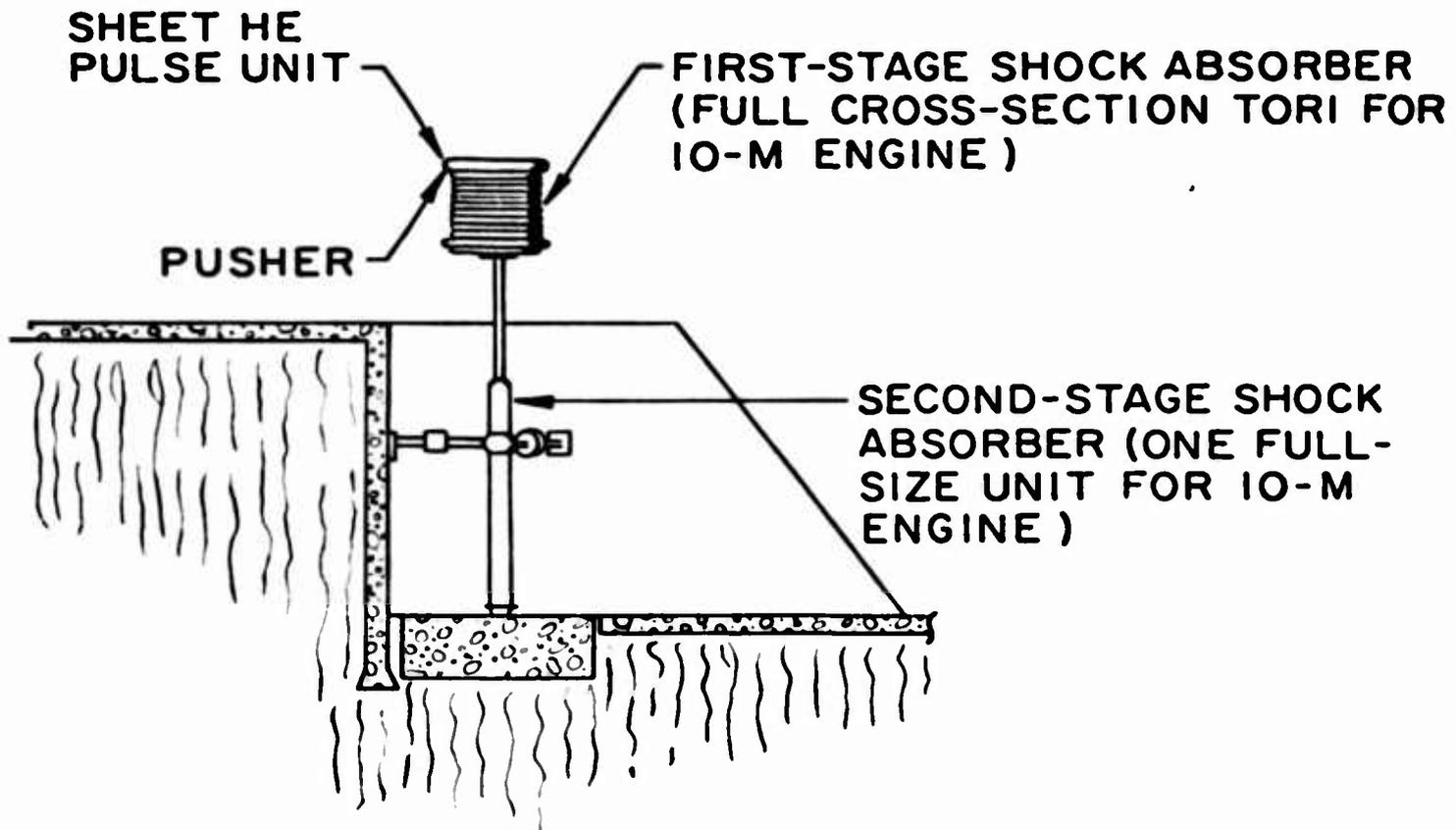
Fig. 8--4-m-diam single-HE-pulse test facility
