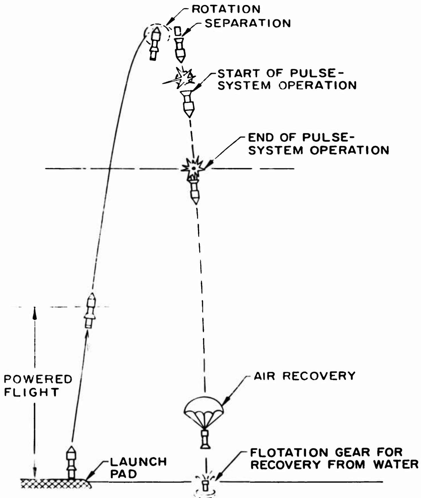
Fig. 11--Trajectory for nuclear ballistic tests
