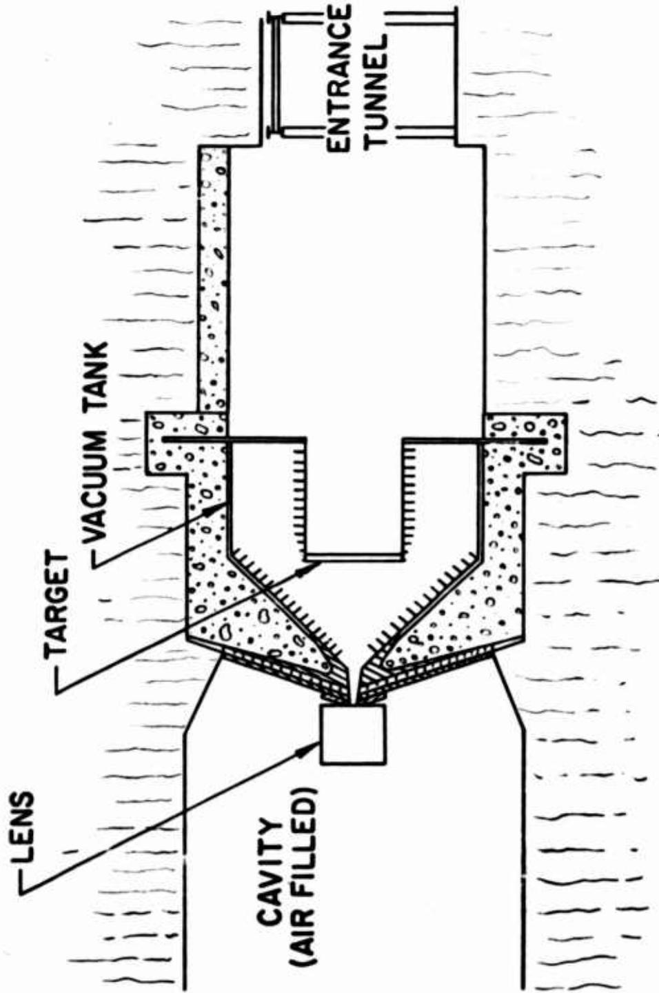
Fig. 10--Underground nuclear test arrangement for propellant-pusher interaction studies
