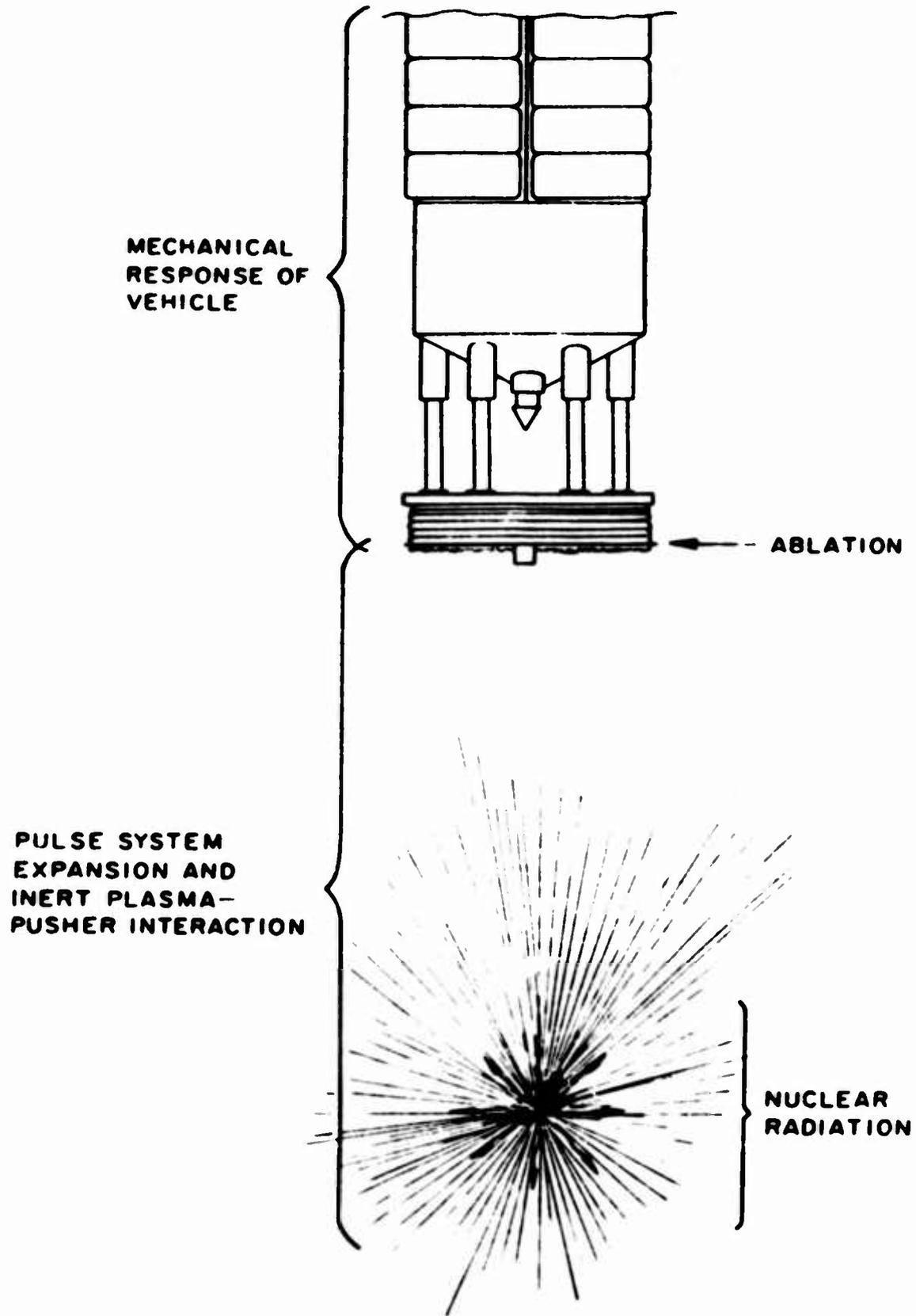
Fig. 2--Separability of nuclear-pulse problems
