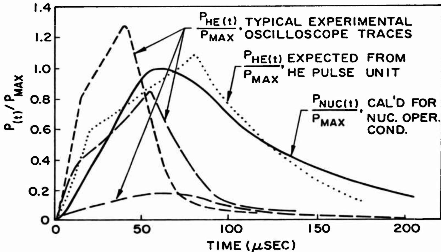
Fig. 4--Pulse shapes for normalized pressure vs time as predicted for nuclear operating conditions and HE test conditions
