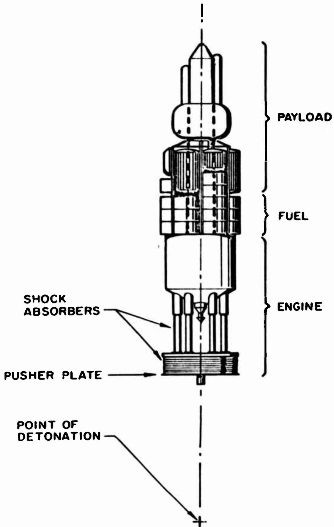
Fig. 1--Reference nuclear-pulse vehicle
