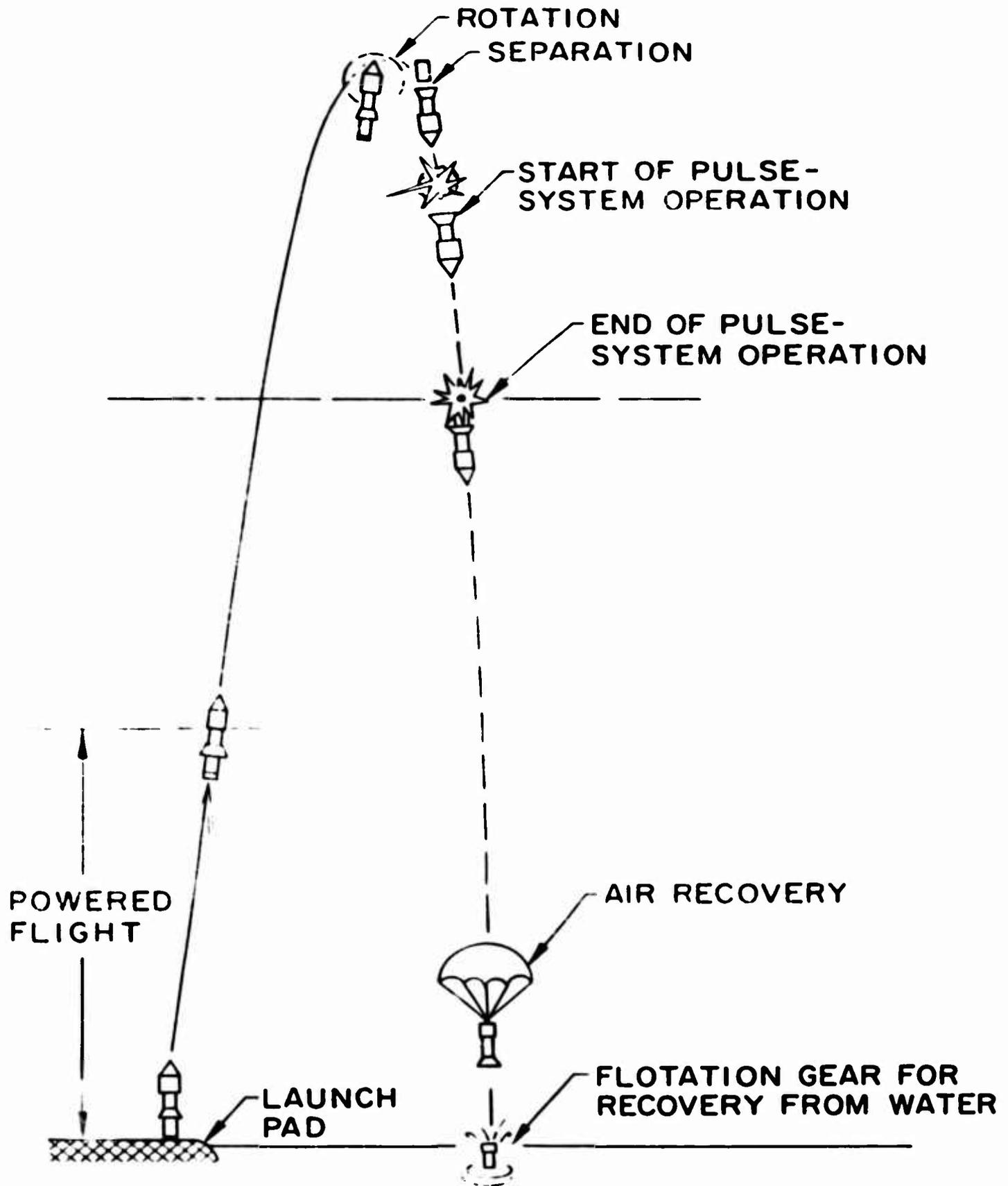
Fig. 11--Trajectory for nuclear ballistic tests
