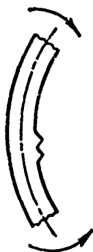
Fig. 4.43. Stability losses in a cylindrical shell with pure bend.
