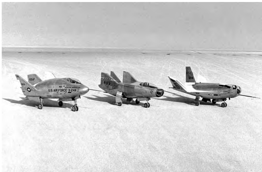
Figure 19: The NASA-Air Force lifting body family in 1969. From left to right are the Martin X-24A, Northrop M2-F3, and Northrop HL-10. The X-24 constituted an Air Force initiative and later spawned the X-24B, which had a much higher fineness ratio. The M2-F3 and HL-10 were “rival” concepts, the former a modified half-cone derived by Ames, the latter a fattened delta derived by Langley. NASA Image E-21093
