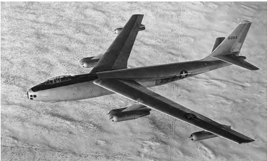
Figure 10: The Boeing XB-47, which introduced the design standard of wing-mounted engine pods combined with a swept-wing planform. Air Force Flight Test Center History Office
