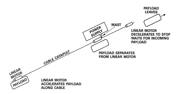
Fig. 3 - The Cable Catapult Concept
