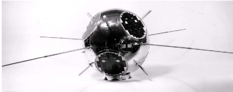
Figure 4. Grab 2 with turnstile antennas
