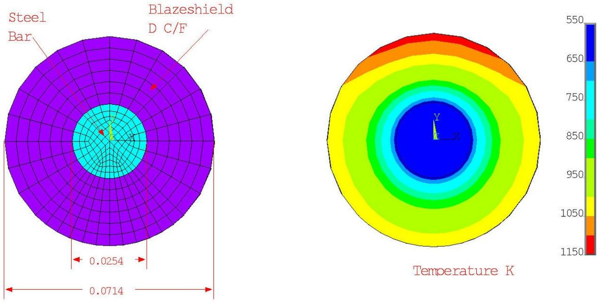
**Figure 5–4. FSI grid structure of insulated steel rod (with dimensions in meters) showing the elements used to model the steel (in blue) and the SFRM (in violet), and the temperature contours after 2,000 s in Test 5.**
