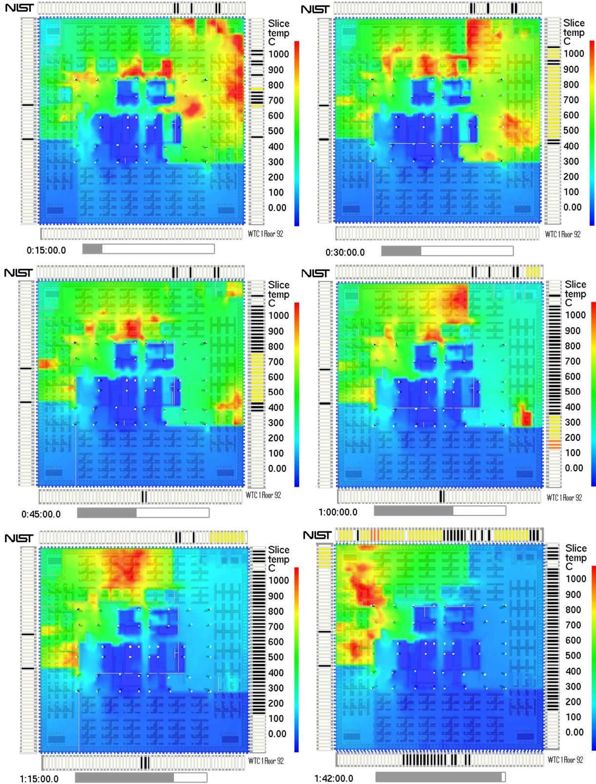
Figure 6–2. Simulated upper layer temperatures on floor 92 of WTC 1, Case B.
