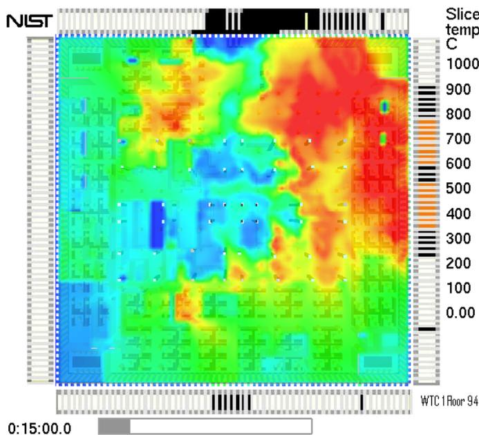
**Figure E–1. Upper layer temperature of WTC 1, floor 94, 15 min after impact.**
