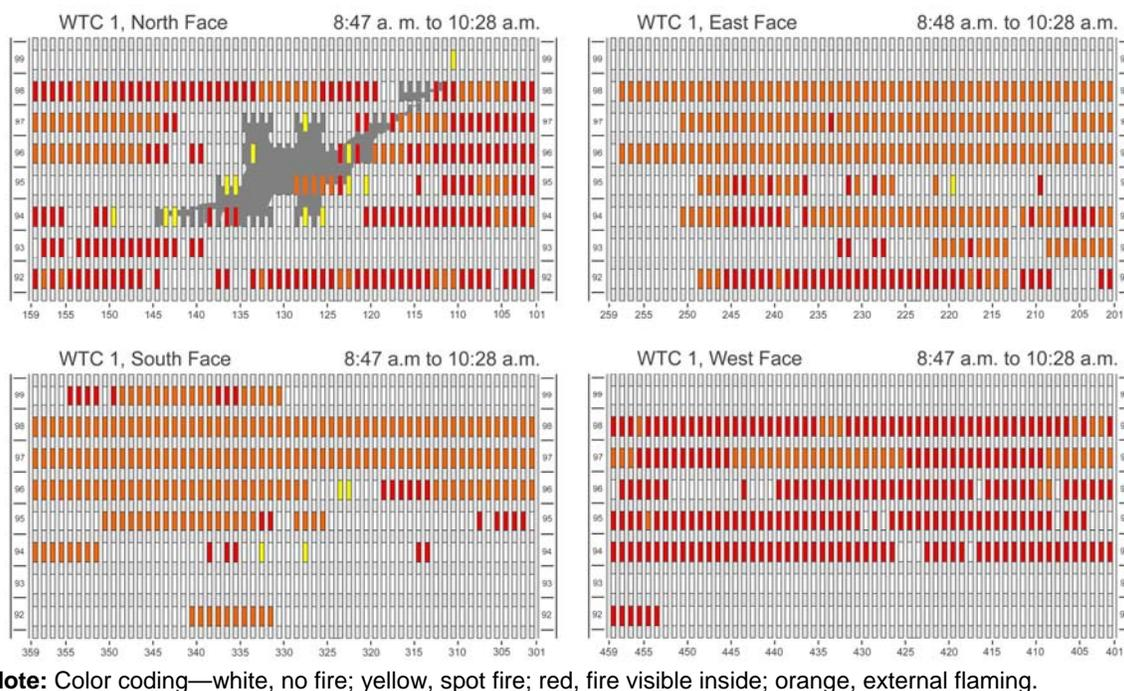
**Figure 2–4. Maps of integrated fire observations between 8:47 a.m. and 10:28 a.m. for the four faces of WTC 1.**
