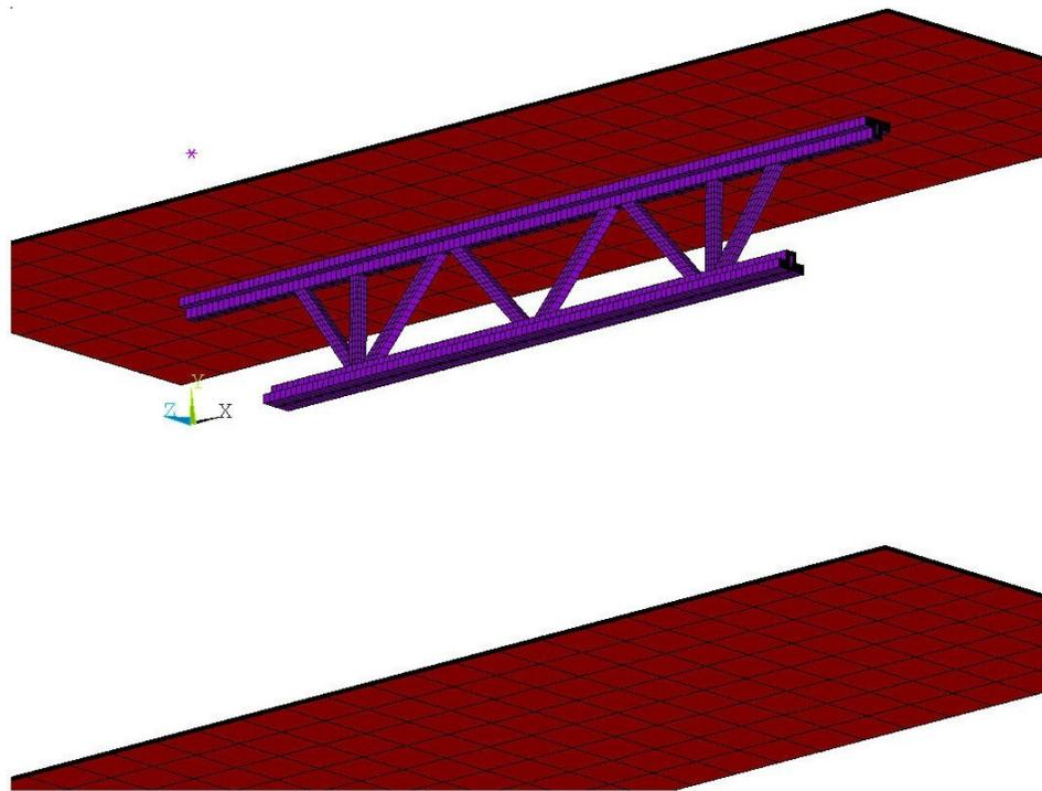
**Figure 5–7. Finite element model of the insulated steel truss, the ceiling and the floor used in the thermal analysis of Test 5.**
