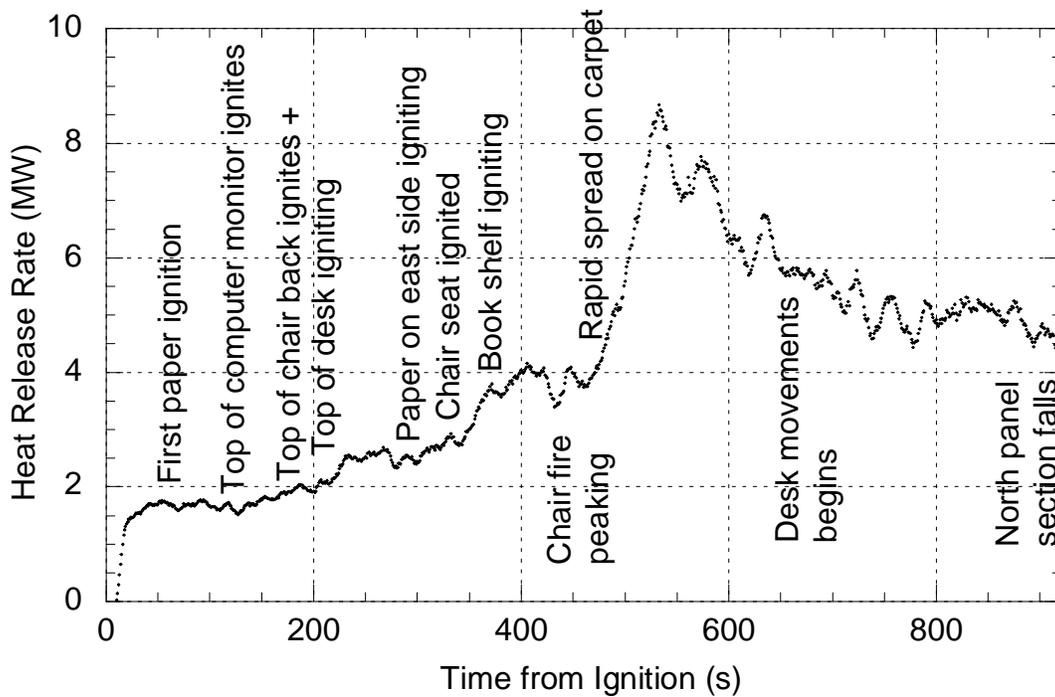
**Figure 3–7. Annotated partial HRR curve from Test 2.**
