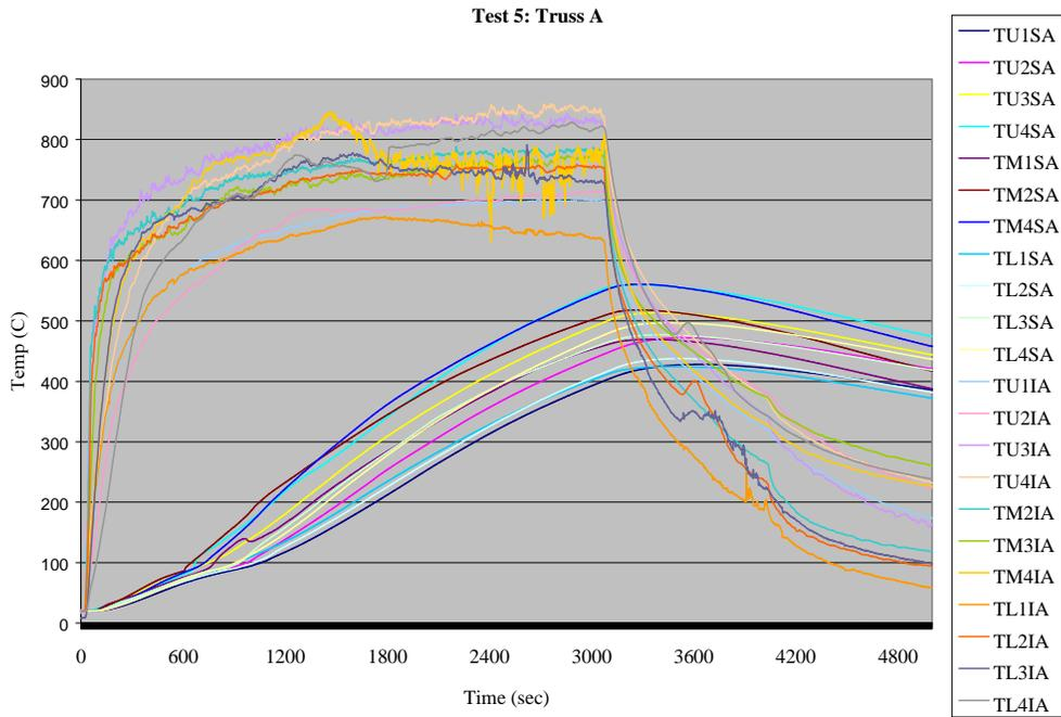
Figure 3–11. Temperature-time history for truss A in Test 5.
