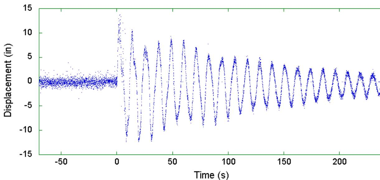
Figure 2-9. Displacement of the left-most window line on the 70<sup>th</sup> floor of WTC 2 as a function of time, determined using Moiré analysis.
