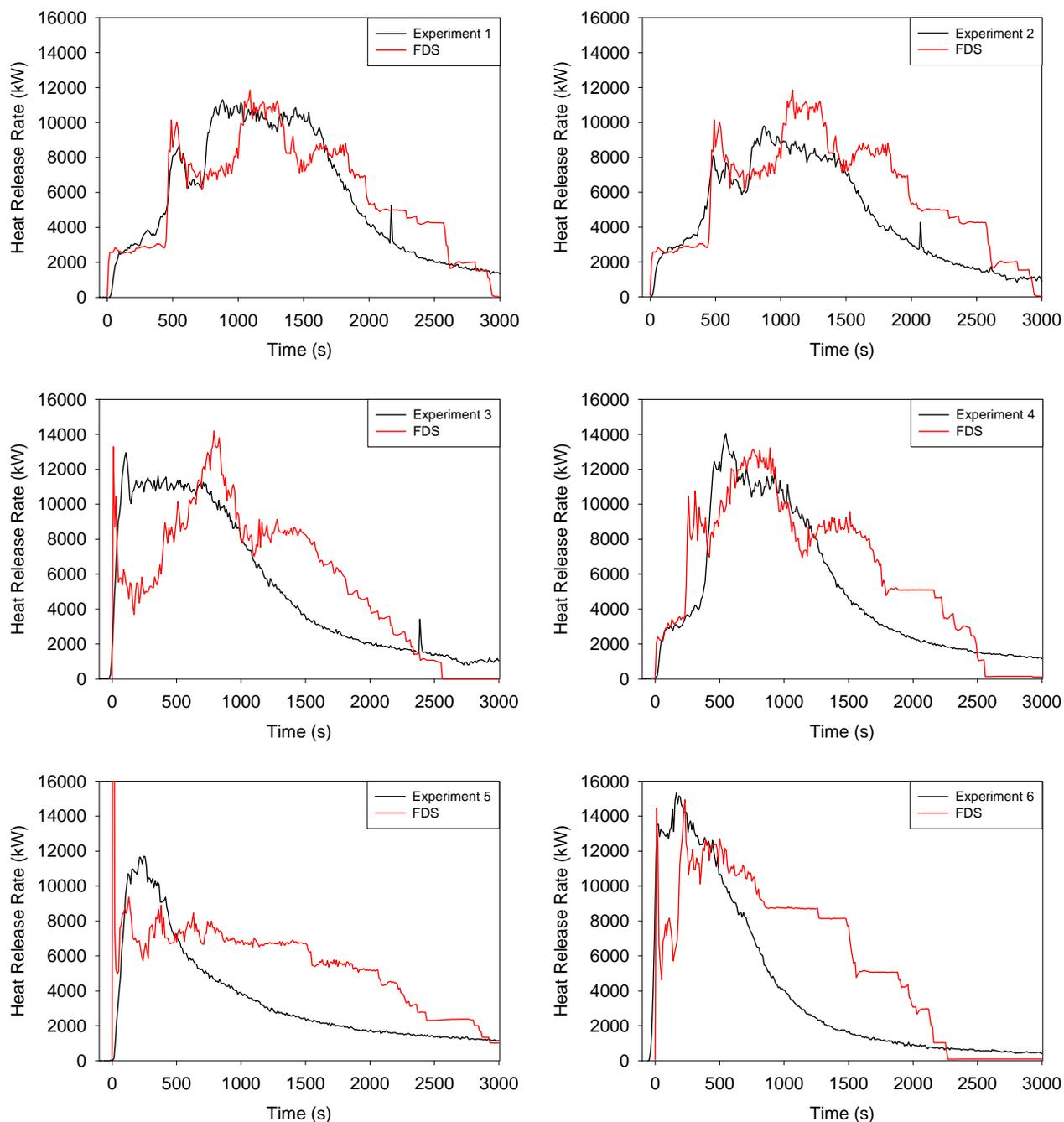
**Figure 4–9. Heat Release Rates for multiple workstation experiments.**
