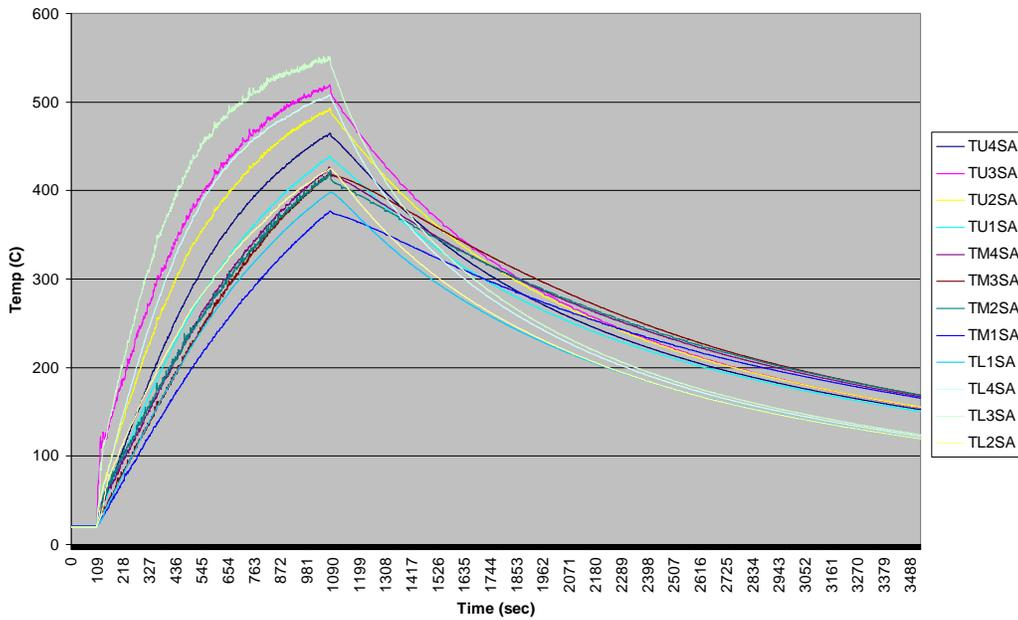
Figure 3–12. Temperature-time history for truss A in Test 3.
