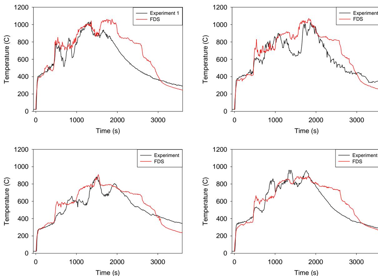
**Figure 4–8. Upper layer temperatures at 4 locations, Test 1.**
