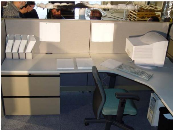
The material make-up of the two workstations is summarized in Table 3–3. The thermophysical properties of both sets of cubicle materials (carpet, desktop, computer monitor, chair, privacy panel, and stacked paper) were determined using the cone calorimeter (ASTM 2003a) for input to the computational simulations. The results of these measurements are given in NIST NCSTAR 1-5C.
