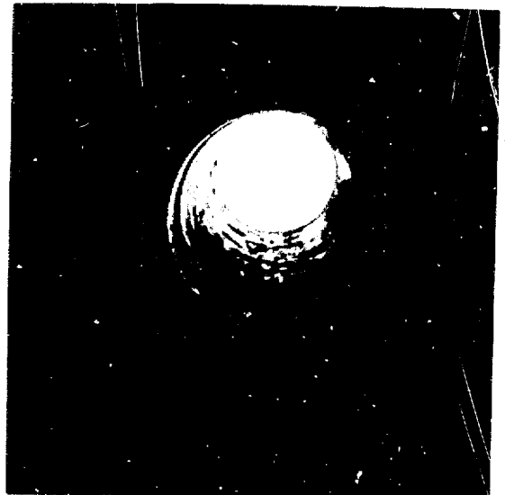
Fig. 1. Glass-lined hole melted in laboratory specimen of tuff.
