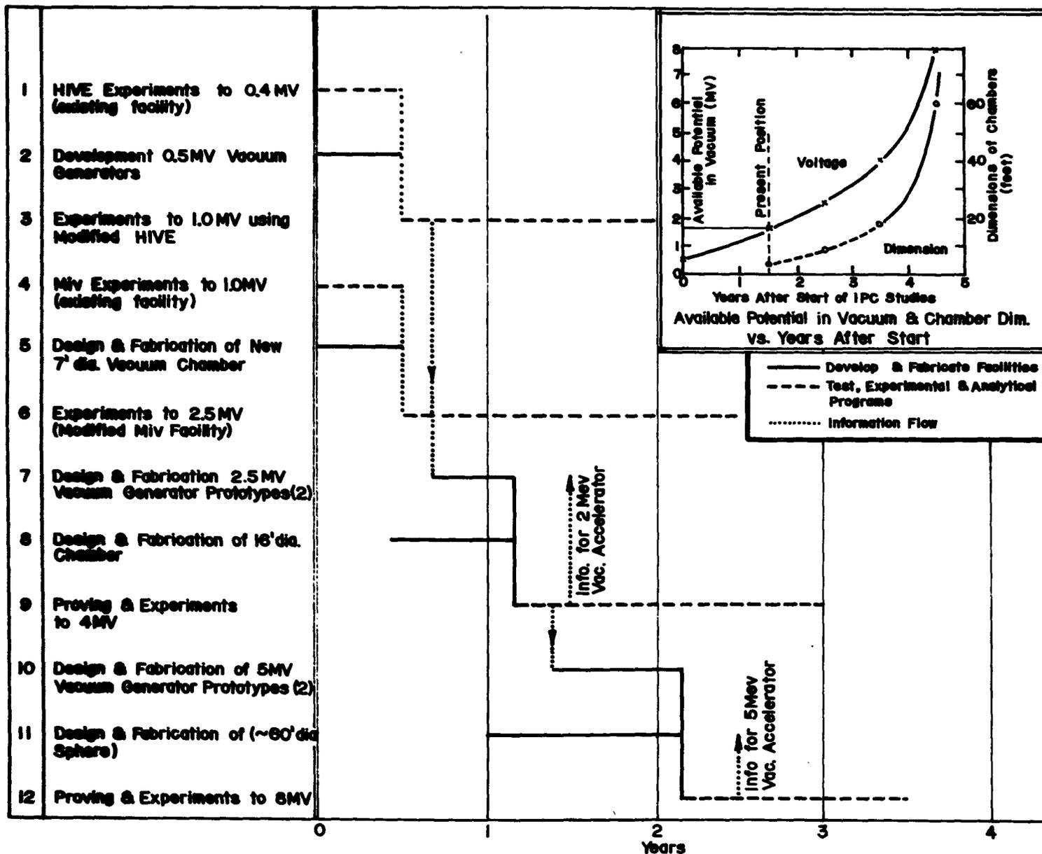
Fig. 39 Growth Plan—High Voltage Insulation Facilities & Studies
