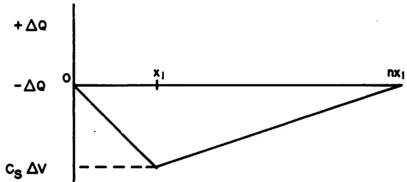
Fig.I-2 Charge Displacement on First Interelectrode Capacitance for 4 Gap Tube. V Position of Charge  $q_p$  Causing Displacement
