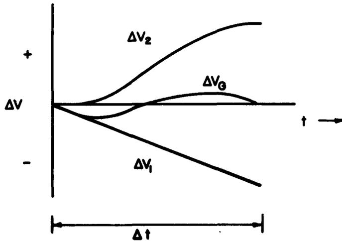
Fig. 6b Voltage Relationships with Resonant Pulsing of Terminal ( $C_2 \gg C_1$ )
