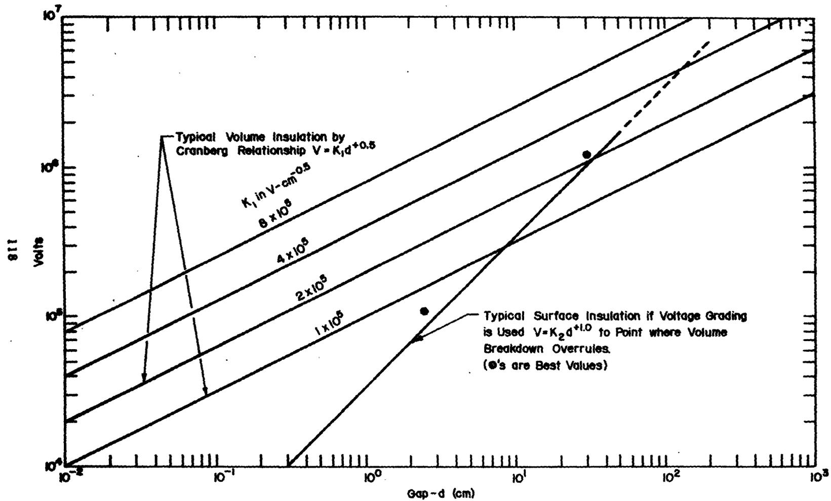
Fig. 28 Voltage-Gap Relationships for Volume and Surface Insulation in Vacuum
