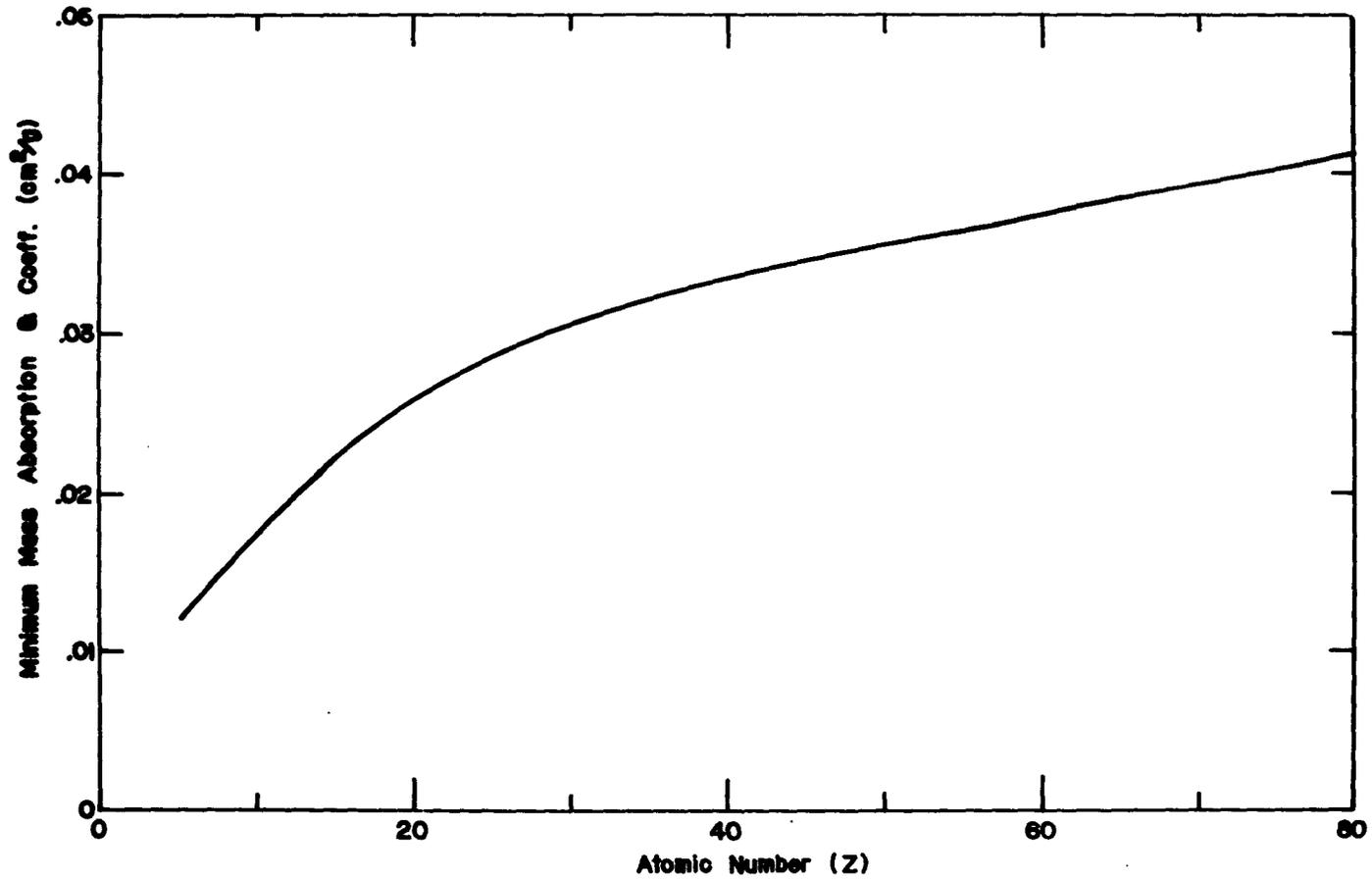
Fig. 17 Absorption Coefficient as a Function of Atomic Number
