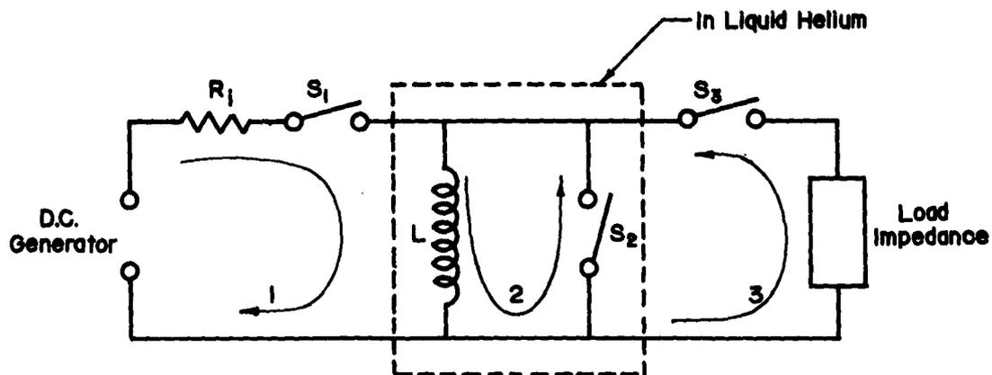
Fig. 8 Superconducting Inductive Energy Storage System
