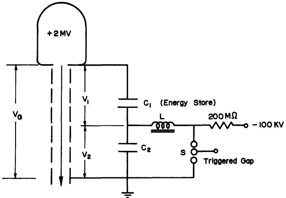
Fig 6a Driven Terminal Concept for Maintenance of Beam Energy During Discharge
