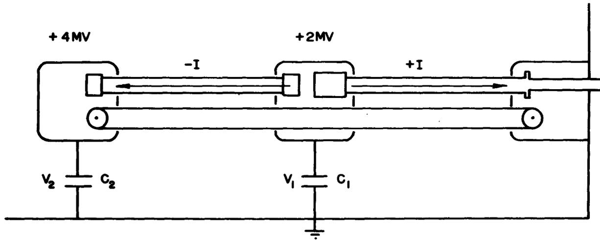
Fig. 7 Maintenance of Beam Energy using an Auxiliary Beam and 2 Terminals.
