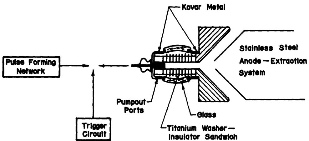
Fig. 10 Occluded Gas Source: Axial Extraction (30)
