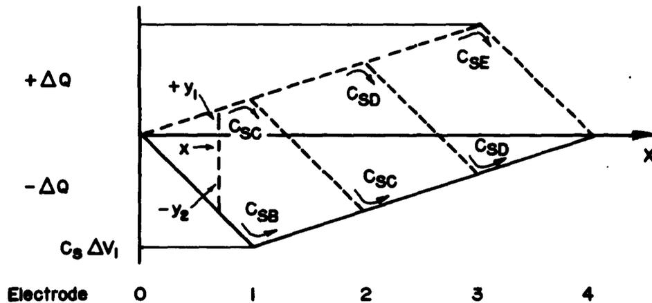
Fig. I-3 Charge Displacement on Each Capacitance V Position of Charge  $q_p$  Causing Displacement
