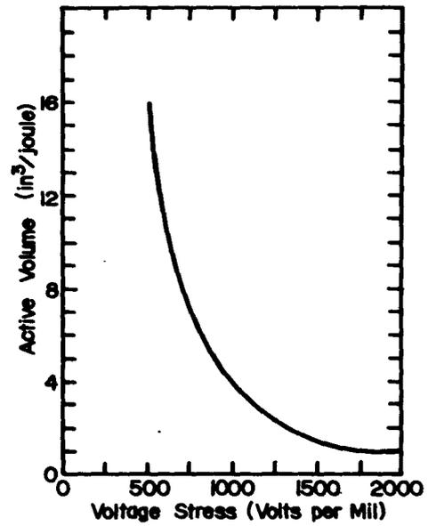
Fig. 4b Energy Density - Stress Relationship for Typical Capacitor Material
