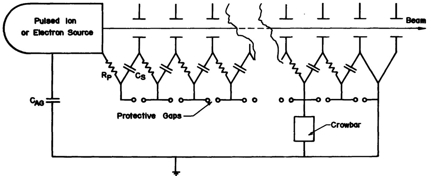
Fig. 2 Circuit Outline - Simple Potential Drop Accelerator
