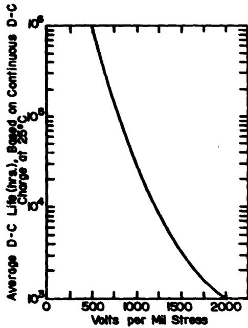
Fig. 4a Life - Stress Relationship for Typical Capacitor Material (Based on 5th Power Law)
