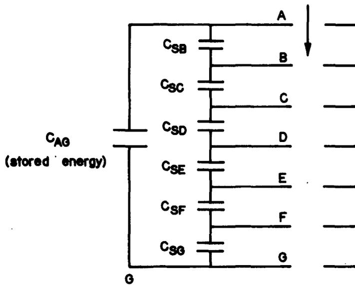
Fig. I-1 Equivalent Circuit - Accelerator Tube System
