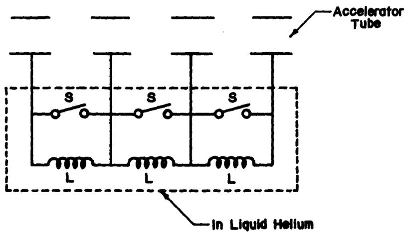
Fig. 9 Coupling of Inductive Energy Storage System to Accelerator Tube
