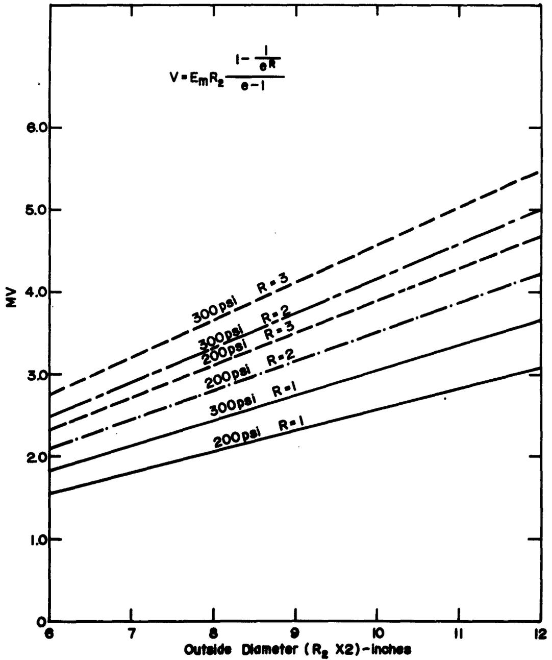
Fig. 36. Voltage Which can be Supported with Cylindrical Geometry Using SF<sub>6</sub>. R is the Number of Coaxial Shells. (Field Data E<sub>m</sub>, Taken from Philp.)
