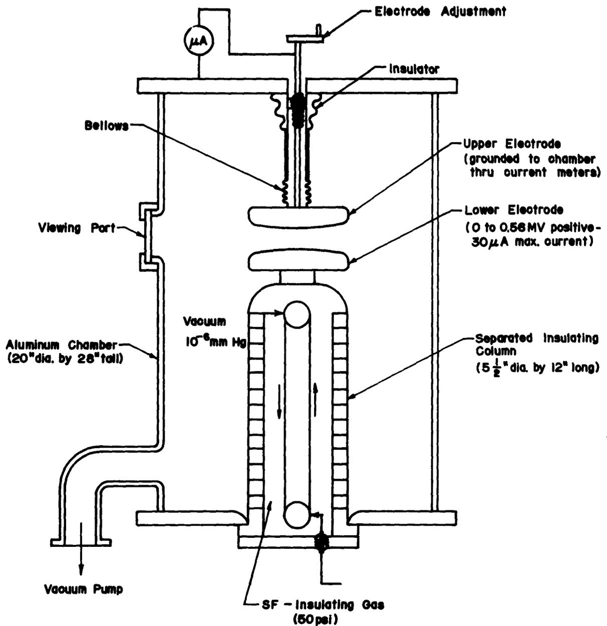
**Fig.30 Conventional Voltage Source, Internally Located
