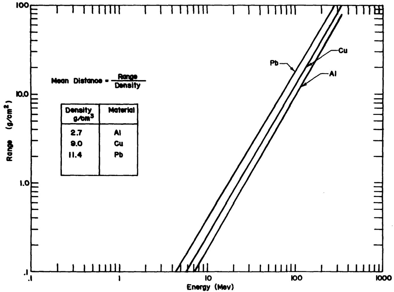
Fig.12 Mean Range of Protons in Metals
