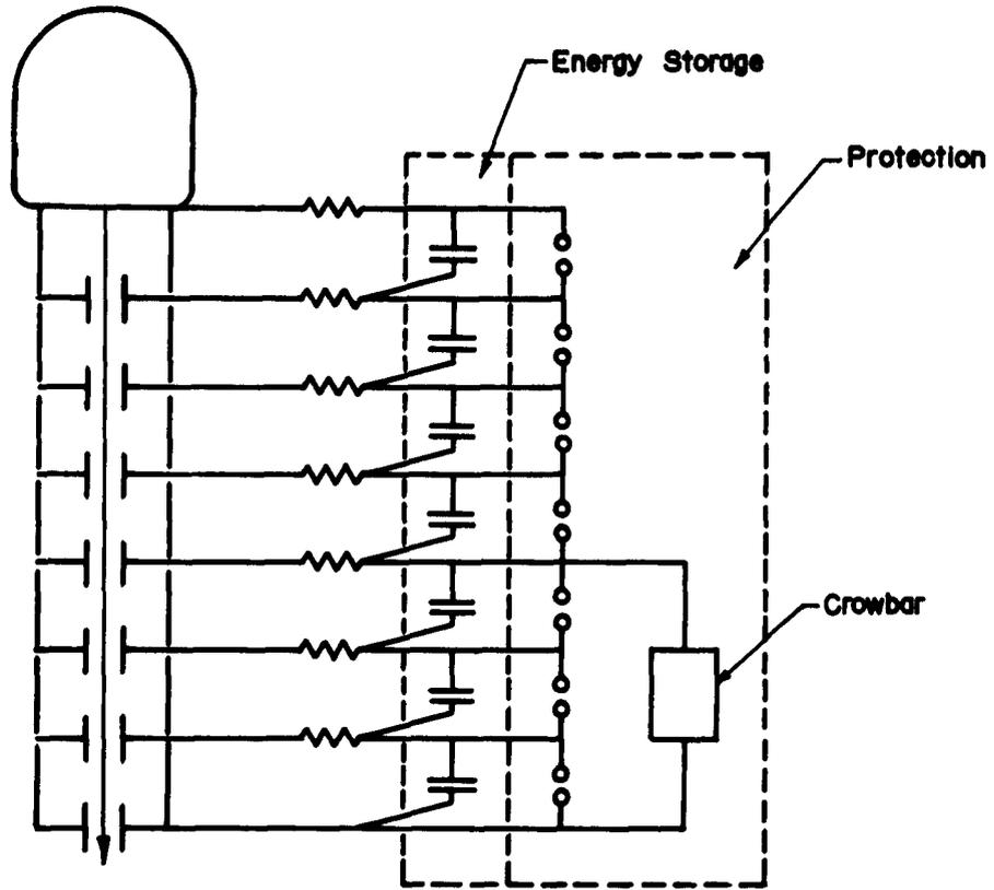
**Fig. 5 Accelerator Coupled for Maximum Beam Stiffness**
