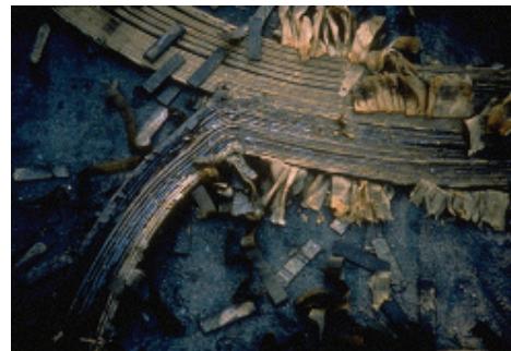
Figure 2-3. GIC Damage to Transformer During 1989 Geomagnetic Storm
