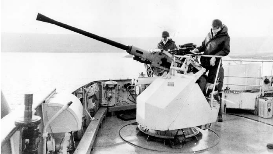
Figure 73. Bofors 40 mm shipboard. In addition to numerous SAMs, the Royal Navy retained guns to protect against air strikes. This Bofors 40 mm L/60 and crew are aboard either the HMS Fearless or HMS Intrepid during the Falklands War. (Reprinted from Imperial War Museum.)
