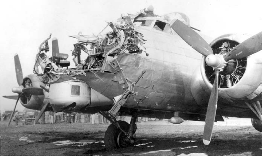
Figure 27. Damaged B-17. This B-17 survived a flak hit over Cologne, Germany. During World War II, the Eighth Air Force suffered 20 percent damage per sortie and wrote off 1,600 bombers as “damaged beyond economic repair.” (Reprinted from USAF.)
