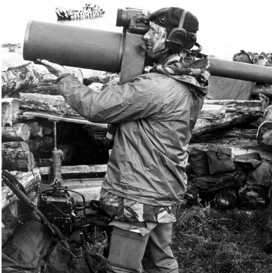
Figure 70. Blowpipe. The British Blowpipe was another shoulder-fired SAM. It was used by both sides in the Falklands War, and both sides claimed it downed aircraft. (Reprinted from Imperial War Museum.)
