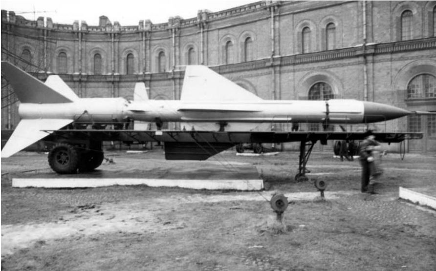
Figure 83. Griffon. The first Soviet ABM known to the West was the Griffon. Flight tests in 1957 led to the construction of 30 firing sites in the early 1960s. But the Soviets stopped construction in 1963 and abandoned the sites the next year. (Reprinted from Federation of Atomic Scientists.)
