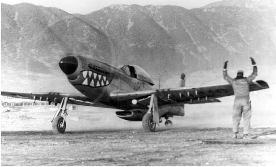
Figure 39. F-51 Mustang. The North American Mustang, the P-51 of World War II fame, saw action as the F-51. It suffered the highest number of USAF losses to enemy action, of which 95 percent of the known losses were to ground fire. (Reprinted from USAF.)
