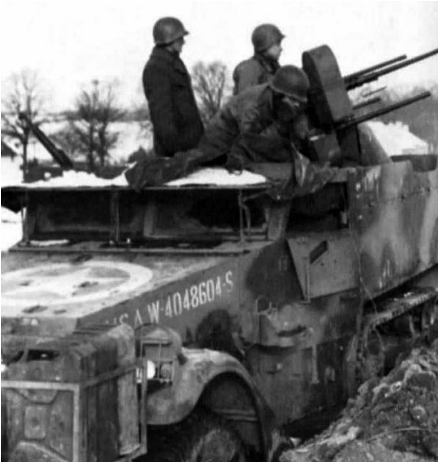
Figure 14. US quad .50 gun. The American quad .50 was an effective weapon against both air and ground targets. (Adapted from http://www.strand.com/quad50/halftrk.jpg .)
