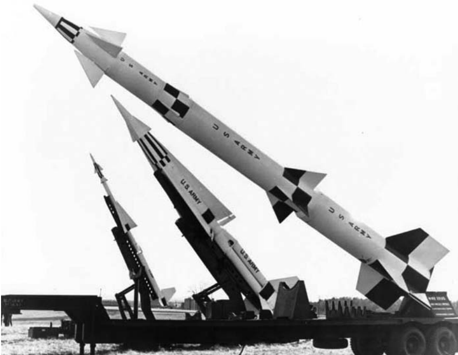
Figure 80. Nike family. America's first ABM family. From right to left (and in the order of their deployment), the Nike Ajax, Nike Hercules, and Nike Zeus. (Reprinted from US Army Aviation and Missile Command.)
