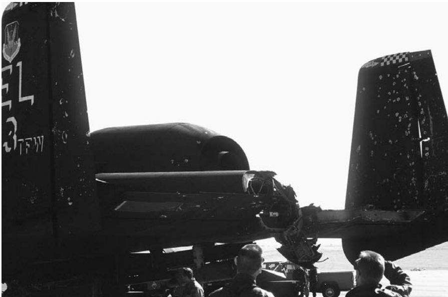
Figure 94. Damaged A-10. Of the 38 coalition air forces lost in combat, only one fell to enemy aircraft. AAA also damaged 24, IR SAMs 15, and radar-guided SAMs four aircraft, including this A-10, one of 13 Warthogs damaged. (Reprinted from Defense Visual Information Center.)
