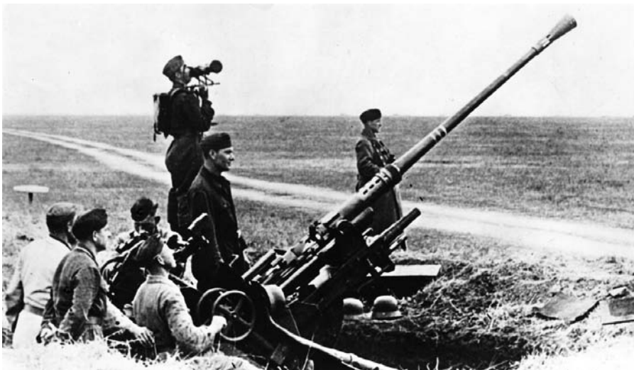
Figure 29. German 20 mm gun. German light flak was very potent. This single 20 mm gun is assisted by the German soldier in the background operating a range finder. (Reprinted from Imperial War Museum.)
