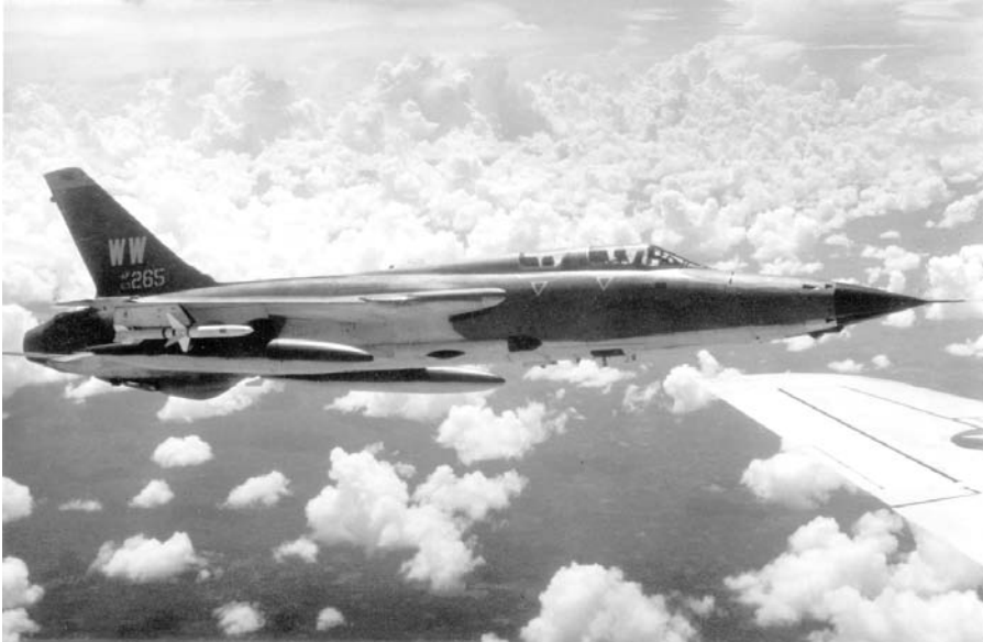
Figure 61. Wild Weasel. The USAF employed special units, called Wild Weasel, to attack Communist radar. This two-seat F-105G is carrying two Shrike antiradiation missiles. (Reprinted from USAF.)
