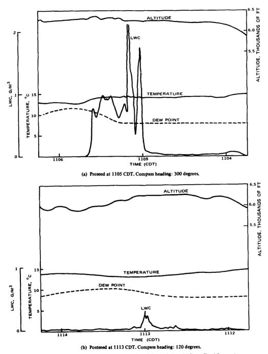
FIG. 3. Liquid Water Content, Temperature, Dew Point, and Altitude, From Cloud Penetrations Versus Time. Increasing time from right to left. Test 11, 25 May 1969. Seed at 1110 CDT.
