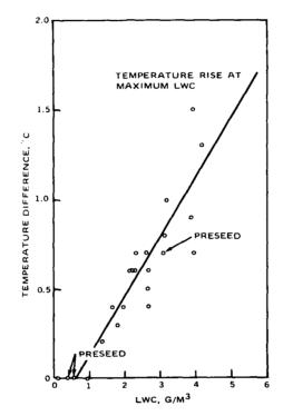
FIG. 8. In-Cloud Temperature Rise Versus Maximum Liquid Water Content. Test 14, 27 May 1969.
