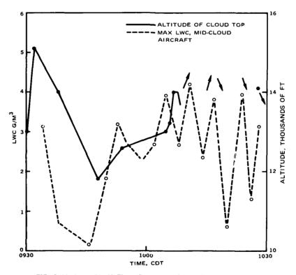
FIG. 5. Maximum Liquid Water Content per Pass and Cloud-Top Altitudes Versus Time. Test 14, 27 May 1969. From 1008 to end of test, arrows indicate direction of growth of cloud based on observer's comments.
