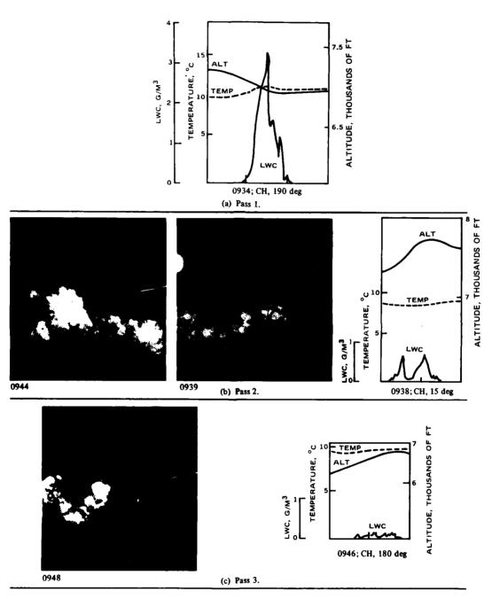
FIG. 4. Liquid Water Content, Temperature, and Altitude Versus Time. Increasing time from right to left. Test 14, 27 May 1969. See Table 3 for explanatory data. Photos from passes 2-7 were taken from approximately 4 nmi: photos from passes 8-15 from approximately 7 nmi. Compass heading (CH) applies to graphs only.
