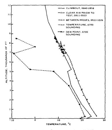
FIG. 6. Temperature and Dew Point Versus Altitude. Test 14, 27 May 1969. Data from 0700 CDT Brownsville sounding and mid-cloud aircraft.
