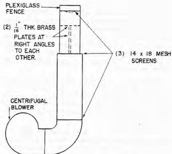
APPARATUS USED TO SUSPEND
