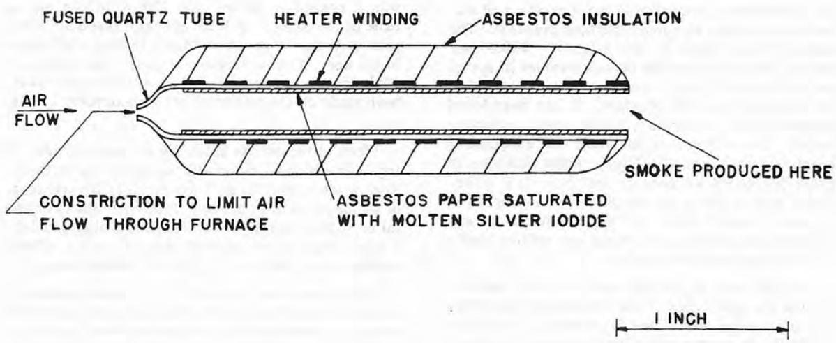
FIG. 3 ELECTRICALLY HEATED GENERATOR
