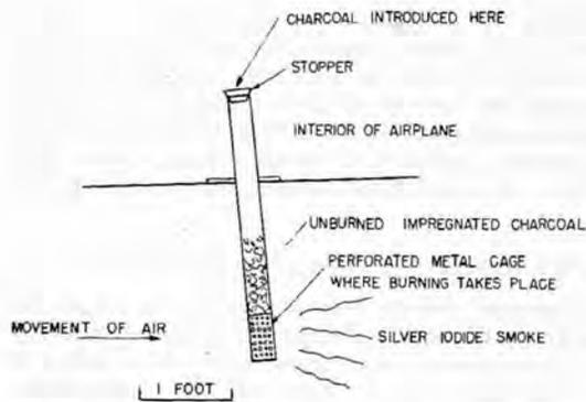
FIG 1 AIRPLANE TYPE SMOKE GENERATOR
