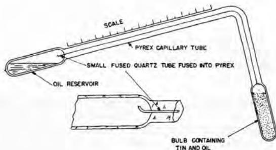
Fig. 2 Dilatometer.
