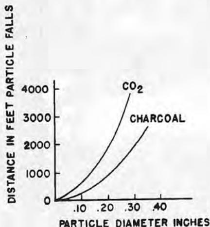
DISTANCE OF FALL OF SOLID CO<sub>2</sub> AND CHARCOAL PARTICLES
