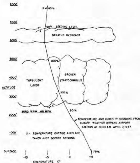
FIG. 8 DIAGRAM SHOWING ATMOSPHERIC CROSS-SECTION APRIL 7, 1947
